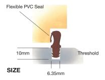
Section size as shown above. Threshold groove size required is 6.35mm (1/4"). Available in standard lengths of 1000mm and 2400mm.
