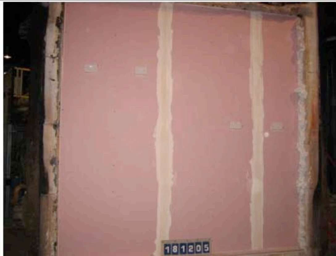
The exposed face of the specimens prior to testing
