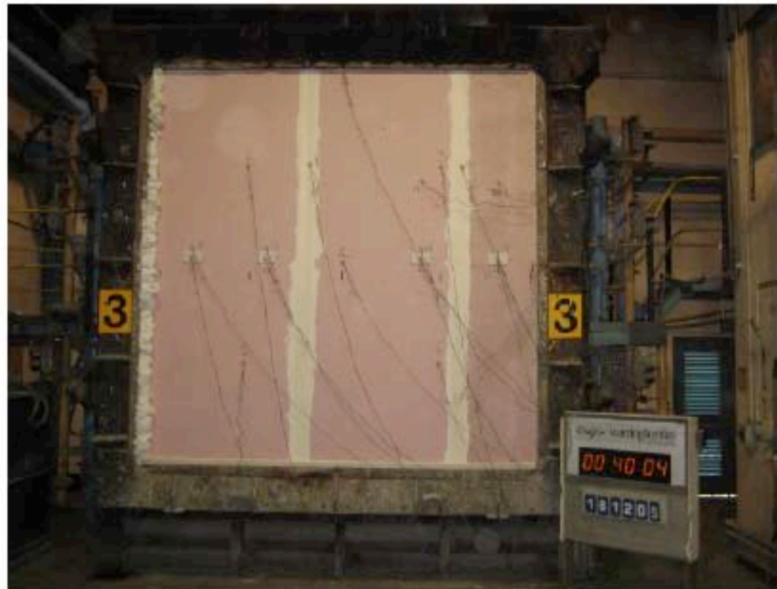
The unexposed face of the specimens after 40 minutes of the test
