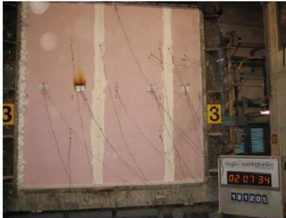
The unexposed face of the specimens after 127 minutes of the test
