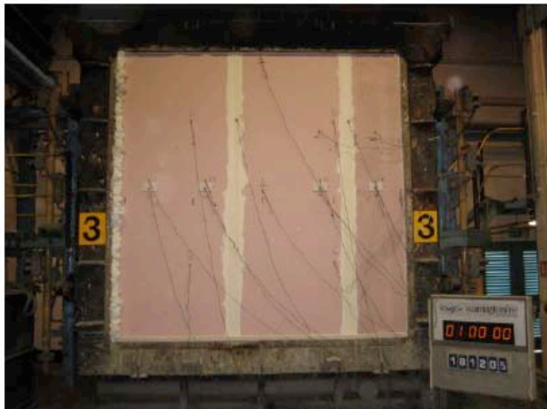
The unexposed face of the specimens after 60 minutes of the test
