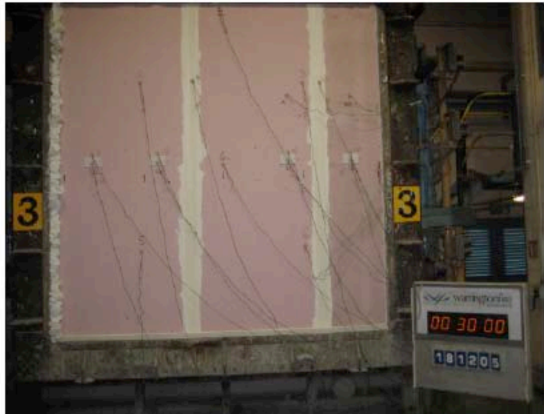
The unexposed face of the specimens after 30 minutes of the test
