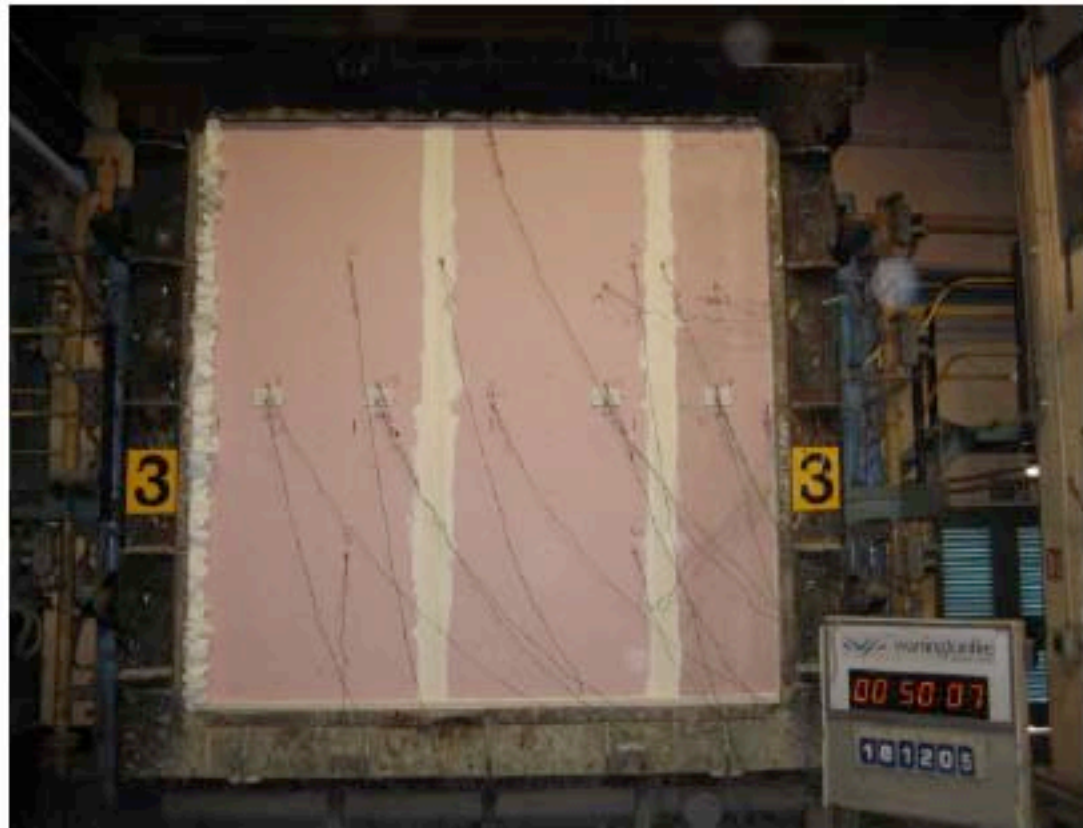
The unexposed face of the specimens after 50 minutes of the test
