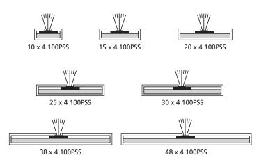
Pyrostrip 100PSS available in depths of 4, 5, 6, 7 and 14mm Widths of 10, 15, 20, 25, 30, 38, 48mm Brush pile in either black or grey, available in 5, 7 or 10mm depths
