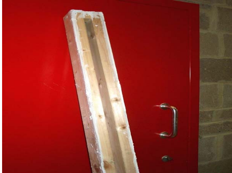
Figure 4 - Sample cassette with 25 mm wide x 100 mm deep open slot
