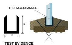
THERM-A-CHANNEL is covered by test report IFCI 290, where a glazed panel 808 x 710mm in a flaxboard core doorleaf, retained by softwood beads attained 36 minutes integrity. Its use in softwood screens is covered by report DIG 9611131 where a softwood screen with central transom attained an integrity rating of 34 minutes.
