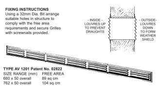
The 1201 Series offers a range of natural ventilation and combustion air grilles for internal and external sidewall and door mounting applications. Manufactured from 0.8mm aluminium sheet the units are supplied mill finish and complete with 2.5 x 24mm spiral pin zinc plated screwnails. The patented 1201 Series was originally designed in conjunction with Mr B J Kipling, Senior Heating Designer of
