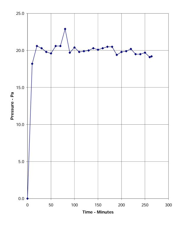
Graph Showing Recorded Furnace Pressure At The Head Of The Upper Row Of Specimens.
