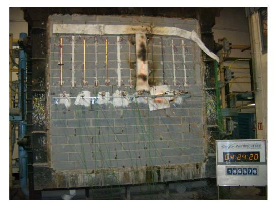
The exposed face of the specimens directly after the test
