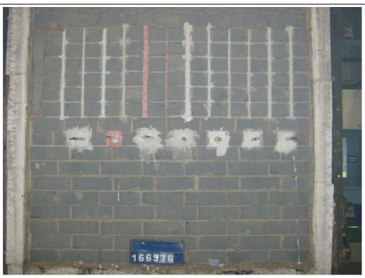
The Unexposed Face Of The Test Construction Prior To Testing
