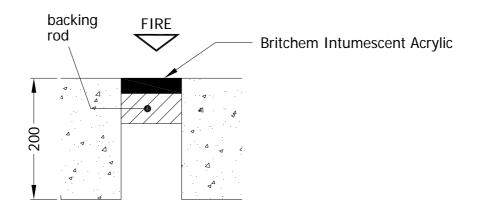
Typical Details for Specimens 'A', 'C' and 'I'
