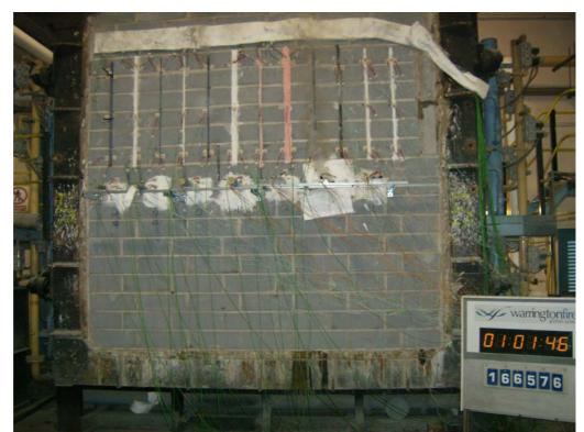
The unexposed face of the specimens after a test duration of 121 minutes
