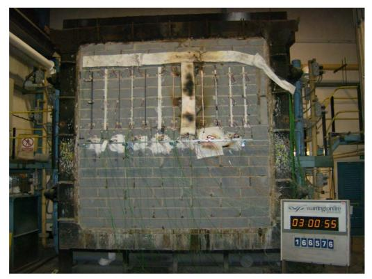
The unexposed face of the specimens after a test duration of 240 minutes
