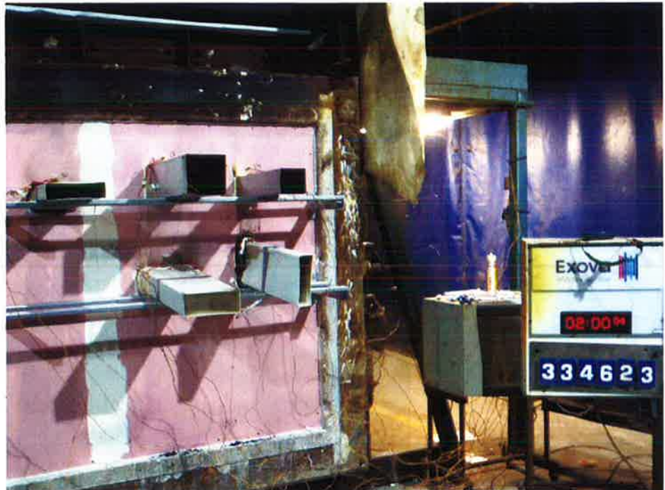
The unexposed face of the test construction after 120 minutes of testing
