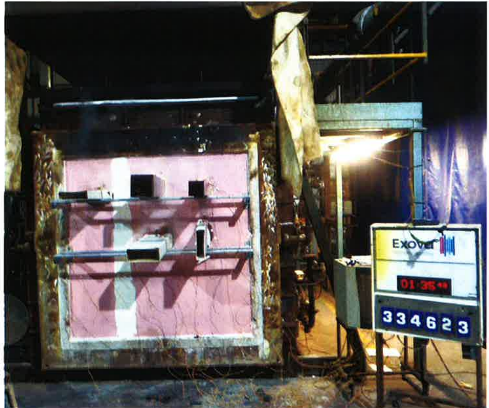
The unexposed face of the test construction after 95 minutes of testing
