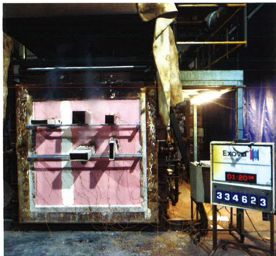
The unexposed face of the test construction after 80 minutes of testing
