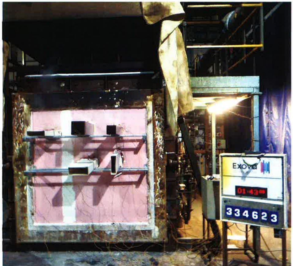
The unexposed face of the test construction after 103 minutes of testing
