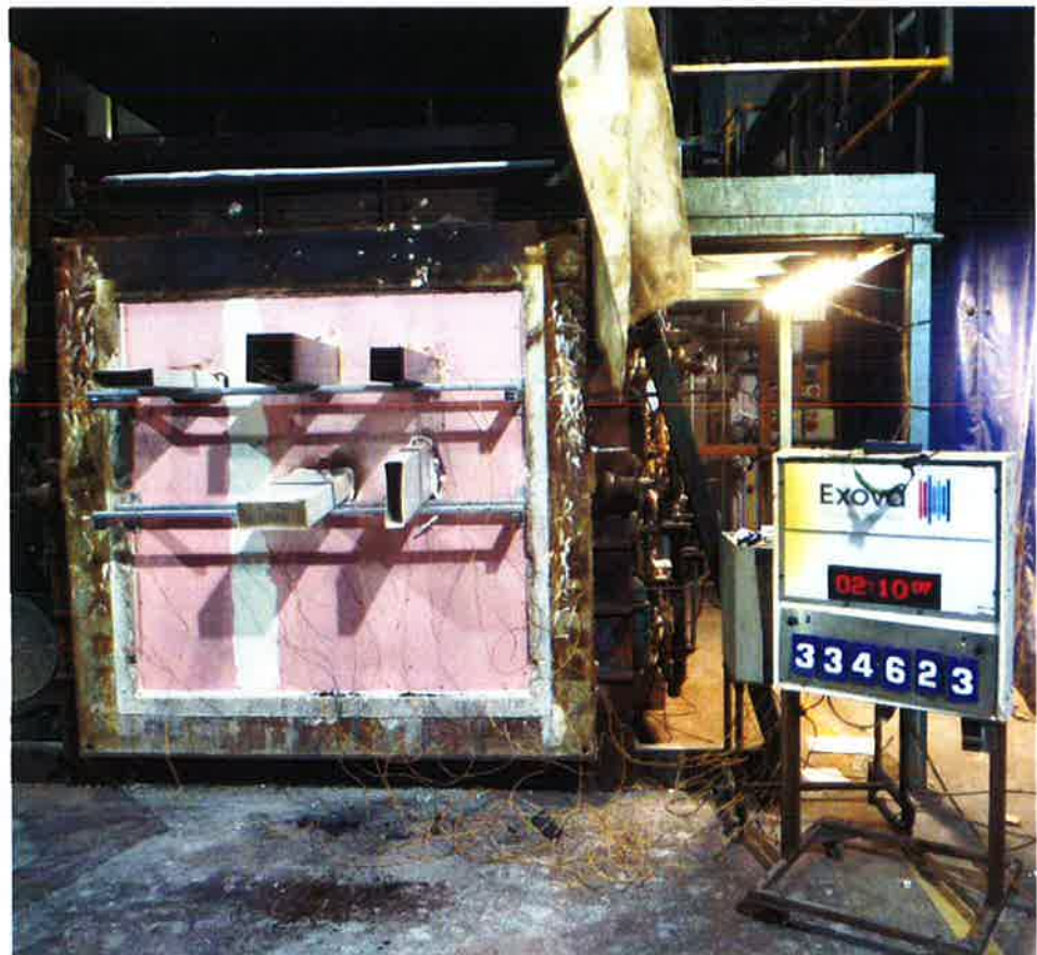
The unexposed face of the test construction after 130 minutes of testing
