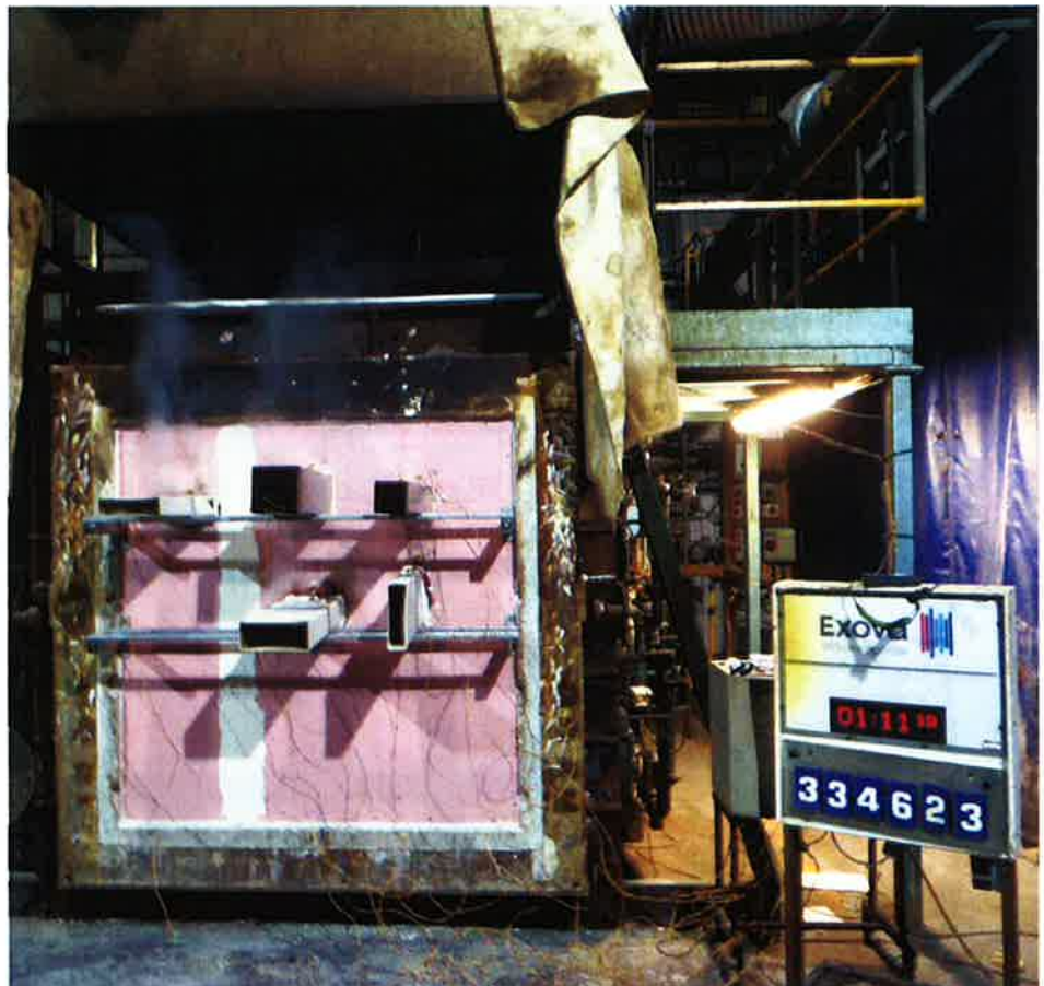
The unexposed face of the test construction after 71 minutes of testing
