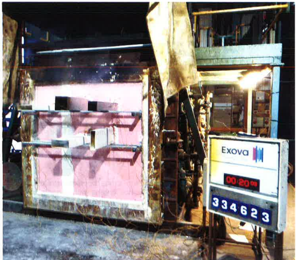
The unexposed face of the test construction after 20 minutes of testing.
